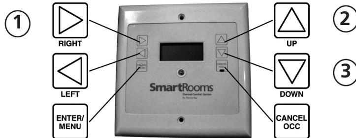
Push the right arrow key first **①** . While holding it down press the up **②** and down **③** arrows at the same time. If successful you will see the message "UPDATED" . If unsuccessful, repeat. The timing of pressing the buttons can be tricky.
