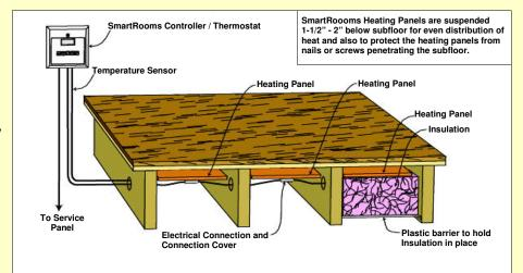
Heating Panels can be suspended by drilling a 1/8" diameter hole through the floor joists and then pull a small gauge wire through the holes and tie off on each end
