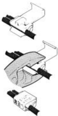
Diagram 2. Connecting the main feed to the individual panel is easily done using tap-on connectors. Note that ONLY the outer insulation jacket of the main feed is removed.
